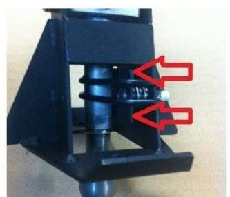
You can also adjust the height of the ball connected to the shift linkage!
