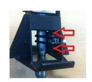
You can also adjust the height of the ball connected to the shift linkage!
